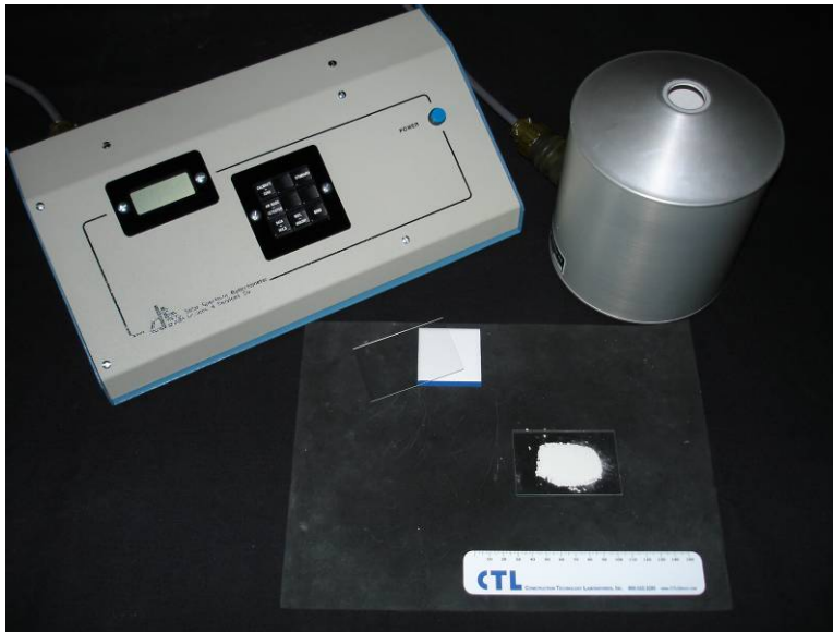
Figure 6. The solar reflectance of a sample of slag cement (white powder on microscope slide near ruler) is measured between two microscope slides (the second slide is lying across the white ceramic tile).
