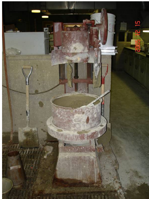
Figure 8. Concrete is mixed in a ½-cubic foot pan mixer.
