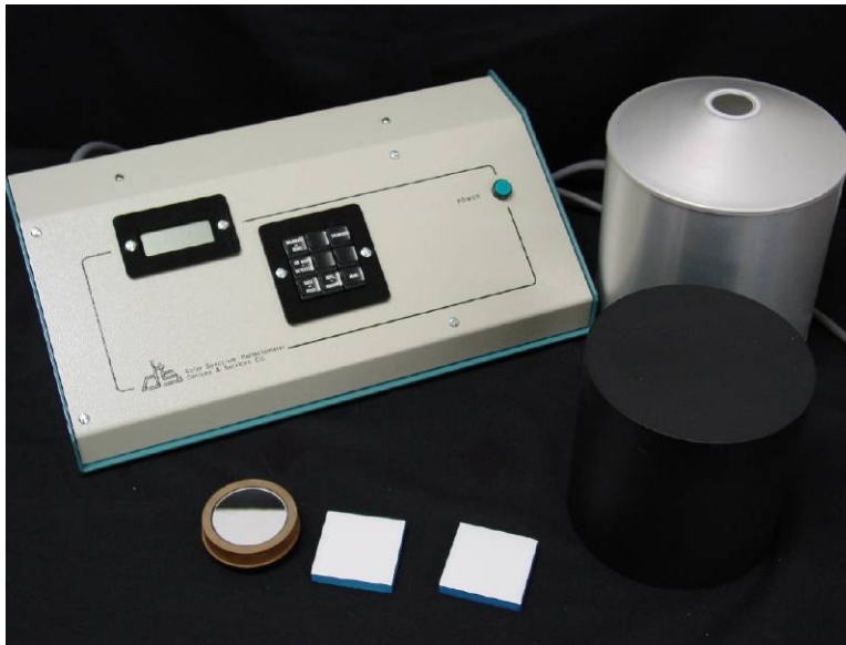
Figure 5. The Devices and Services Company solar spectrum reflectometer model SSR-ER is shown with the measurement head (upper right), black body cavity (lower right), and three calibration standards (a round mirror, and two square white ceramic tiles).
